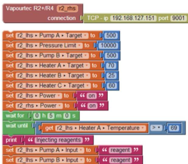
Fig. 1 Example of automated experiment using Blocktopus user interface.
