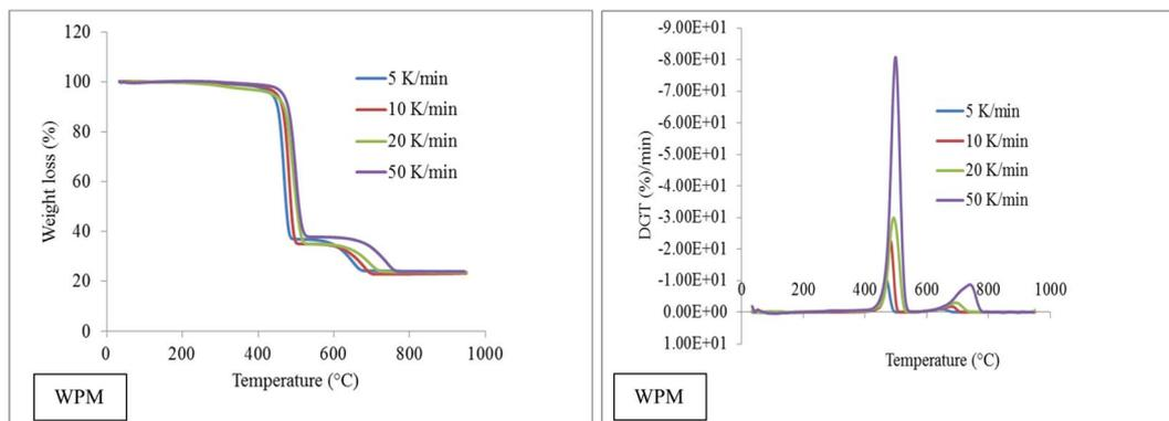
Fig. 2 Plots of TGA and DTG of WPM.
