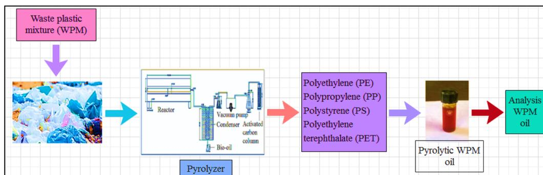
Fig. 4 Schematic diagram of the pyrolysis process set-up for slow pyrolysis.
