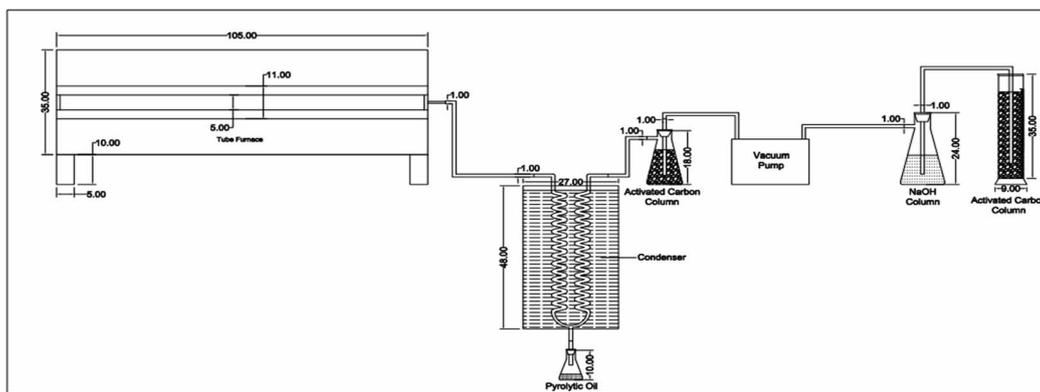
Fig. 1 Schematic diagram of pyrolytic oil set-up (ref. 50).
