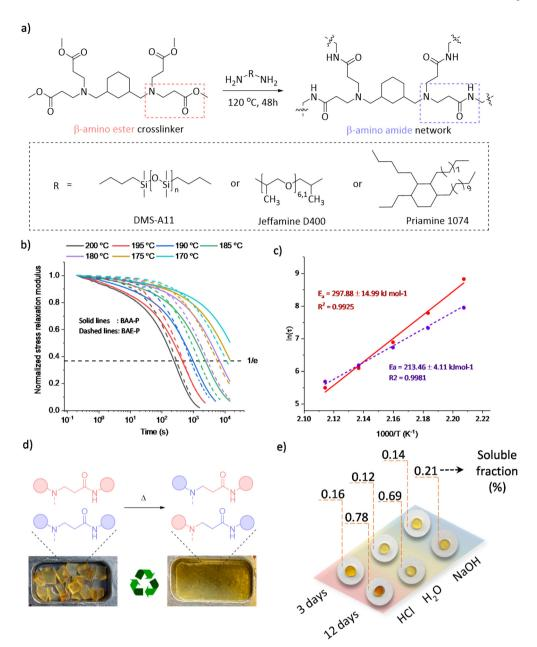
Fig. 4 (a) Preparation of β-amino amide containing CANs from a tetrafunctional crosslinker and Priamine 1074 (BAA-P), Jeffamine D400 (BAA-J) or DMS-A11 (BAA-S); (b) normalized stress relaxation curves and (c) corresponding Arrhenius plots of BAA-P (red) and BAE-P (violet) networks; (d) demonstration of (re)processing of BAA-P; (e) appearances and the corresponding soluble fractions of BAA-P samples after the hydrolysis tests under different conditions (1 M HCl, deionized water, 1 M NaOH).
