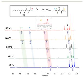
Fig. 2 <sup>1</sup>H NMR stacking spectra of model compound 1 in DMSO-d<sub>6</sub> at 25 °C, 120 °C, 140 °C, 160 °C and 180 °C for 16 h.
