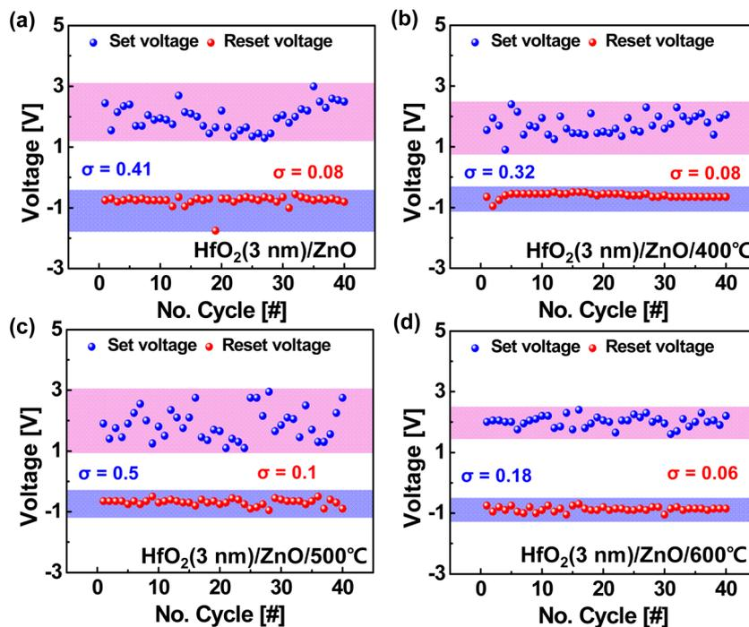
Fig. 6 Obtained VSET and VRESET distributions for 40 consecutive  $I$ – $V$  sweeps for bilayer  $\text{HfO}_2/\text{ZnO}$  synaptic devices (a) without and with thermal annealing at (b) 400 °C, (c) 500 °C, and (d) 600 °C.
