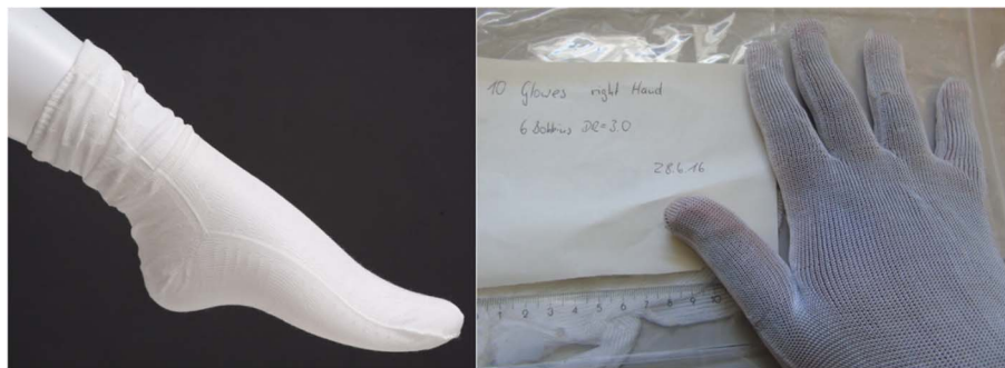
Fig. 10 Images of a sample repellent sock and glove made from porous polymeric materials. Reproduced from ref. 97 with permission from Elsevier, copyright 2018.
