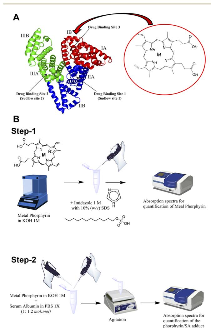
**Scheme 1** (A) Schematic illustration of the interaction of serum albumin with protoporphyrin IX ( $M = \text{Mn(III)}$  or  $\text{Fe(III)}$  or  $\text{Zn(II)}$ ). (B) Scheme of the preparation of metal porphyrin serum albumins (step-1: UV-vis spectrophotometric quantification of metal porphyrin; step-2: preparation and quantification of metal porphyrin serum albumins).
