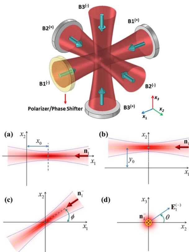
**Fig. 1** Schematic diagram of the proposed setup (top diagram) as well as defining the parameters of beam  $1^{(-)}$  used in the simulations. (a) Axial offset ( $x_0$ ), (b) lateral offset ( $y_0$ ), (c) propagation direction of beam  $1^{(-)}$  with respect to the  $x_1$  axis ( $\phi$ ), and (d) polarization direction of beam  $1^{(-)}$  from the  $x_2$  axis ( $\theta$ ).
