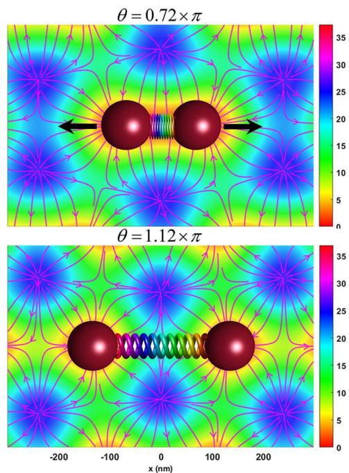
Fig. 6 DNA stretching or compressing with dynamic lattices generated by adjusting the polarization state of beam  $1^{(-)}$ . The streamlines show the optical force field lines on the  $xy$  plane, and the colorbar values indicate normalized potential energy profile in the  $xy$  plane. An animation of DNA stretching and compressing is also given in visualization 7.†
