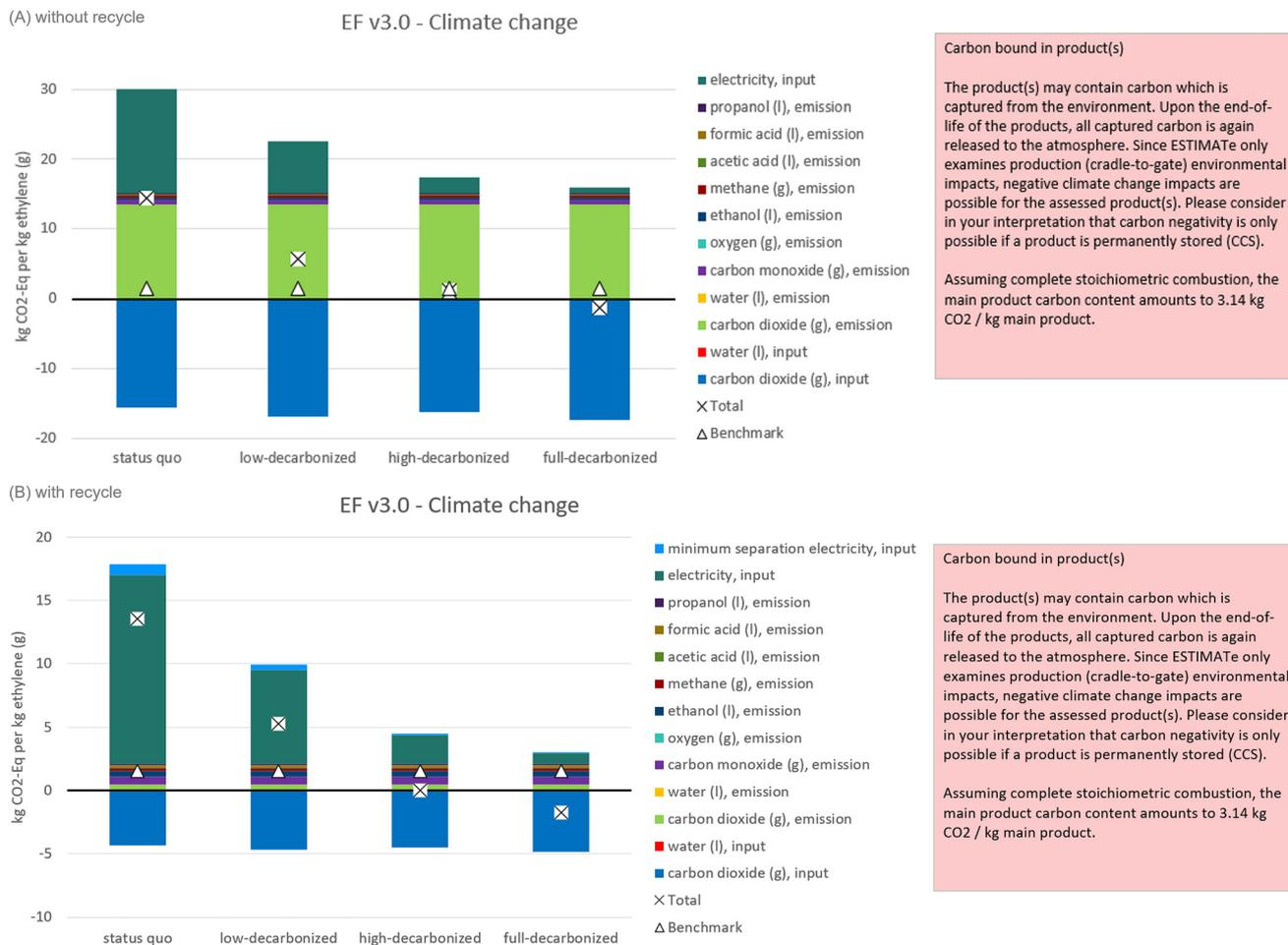
**Fig. 5** Climate Change Impact of laboratory-scale electrochemical CO<sub>2</sub> reduction to ethylene in the ESTIMATE tool. (A) Without recycle of unreacted CO<sub>2</sub>, (B) including a recycle of unreacted CO<sub>2</sub>. Note the different scales of the y-axes. The different bars correspond to the different background system scenarios defined in section 2.4.
