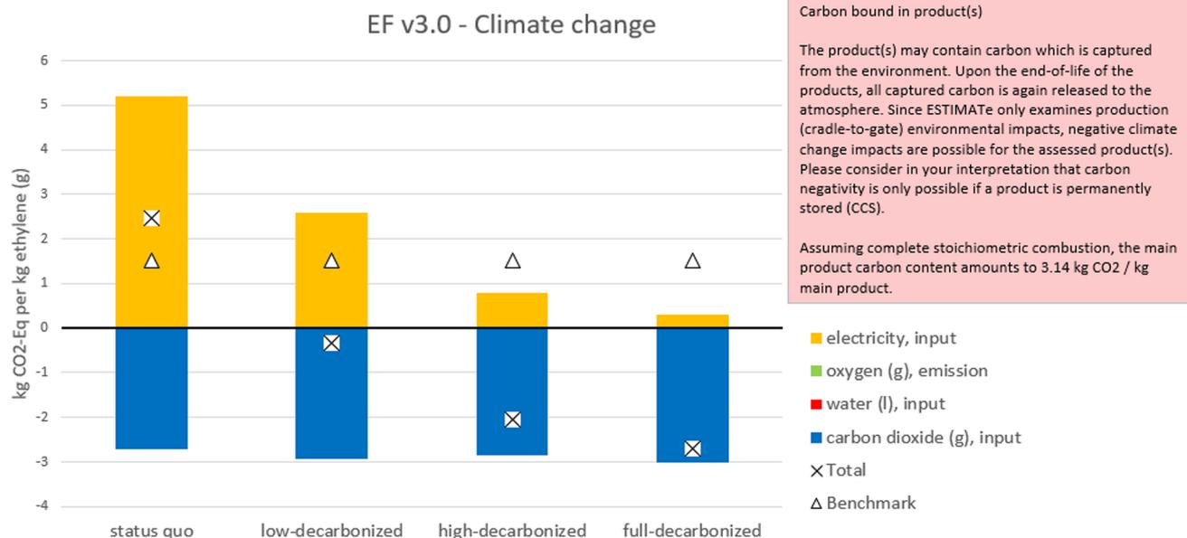
**Fig. 3** Climate Change Impact of the Best-Case Assessment of electrochemical CO<sub>2</sub> reduction to ethylene in the ESTIMATE tool. The different bars correspond to the different background system scenarios defined in section 2.4.
