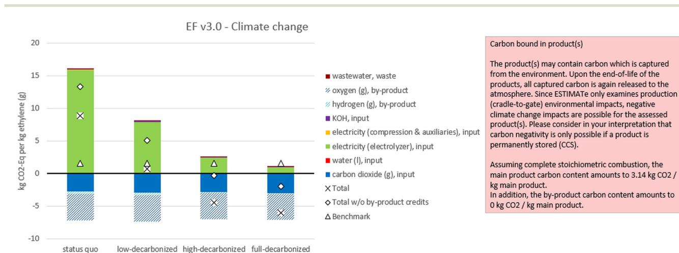
**Fig. 6** Climate Change Impact of process-design-scale electrochemical CO<sub>2</sub> reduction to ethylene calculated by the ESTIMATE tool. The different bars correspond to the different background system scenarios defined in section 2.4.
