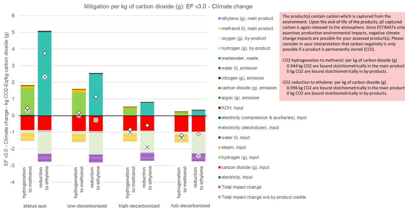
**Fig. 8** Climate Change Impact results of the Mitigation Potential Assessment comparing electrochemical CO<sub>2</sub> reduction to ethylene (left bars) and CO<sub>2</sub> hydrogenation to methanol (right bars) in the ESTIMATE tool. The different bar clusters correspond to the different background system scenarios defined in section 2.4.
