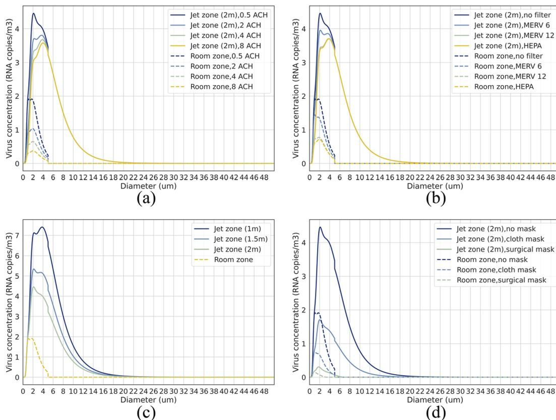
Fig. 3 Droplet size-dependent virus concentration in the jet zone (within a distance of 2 m from the infector (solid line)) and room zone (with a distance of >2 m from the infector (dashed line)) with different control strategies of: (a) ventilation; (b) filtration; (c) distancing; (d) masks.
