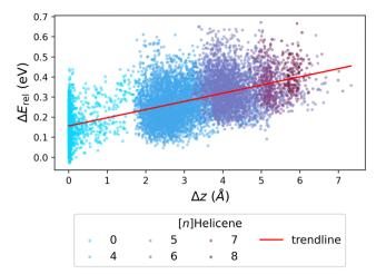
Fig. 7 Scatter plot of  $\Delta E_{\rm rel}$  vs.  $\Delta z$ , colored by the longest [n]Helicene present in the molecule (0 indicates no helicene motifs). The red line shows the trendline of the data
