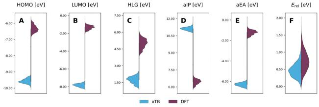
Fig. 5 Violin plots of xTB-calculated (blue) properties vs. DFT-calculated (purple) properties: (A) HOMO; (B) LUMO; (C) HLG; (D) aIP; (E) aEA; (F) E<sub>rel</sub>. All values are reported in eV.
