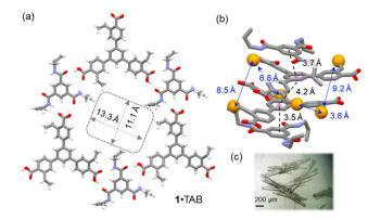
Fig. 1 (a) Single-crystal structure of the  ${\bf 1}$ -TAB co-crystal viewed along the b/c plane. (b) The ABBA-type alternative packing of  ${\bf 1}$  and TAB, viewed along the a-axis. The  $\pi$ - $\pi$  stacking distances and distances between the terminal carbon atoms of the styrene moieties are highlighted. (c) An image of  ${\bf 1}$ -TAB co-crystals.
