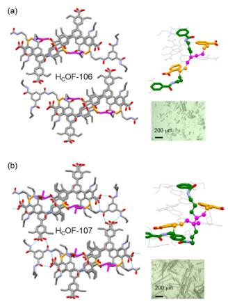
Fig. 3 The SCXRD structure of (a)  $H_COF-106$  and (b)  $H_COF-107$  with highlighted crosslinkers (magenta) in the crystal lattices. The crosslinking connections between the layers in H<sub>C</sub>OF-106 and H<sub>C</sub>OF-107 are shown on the right. Inset: Optical images of these crystals.
