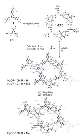
Scheme 1 Synthesis of  $H_{C}OF-106$  and  $H_{C}OF-107$  through free-radical reactions with butadiene and isoprene. Post-modification of the single-crystalline  $H_{C}OF-107$  affords its hydroxylated derivative  $H_{C}OF-108$ .
