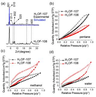
Fig. 4 (a) Simulated (H<sub>C</sub>OF-107) and experimental PXRD patterns of  $H_{C}OF-107$  and  $H_{C}OF-108$ . (b) Pentane, (c) methanol, and (d) water vapor sorption isotherms (295 K) for H<sub>C</sub>OF-107 (black) and H<sub>C</sub>OF-108 (red).
