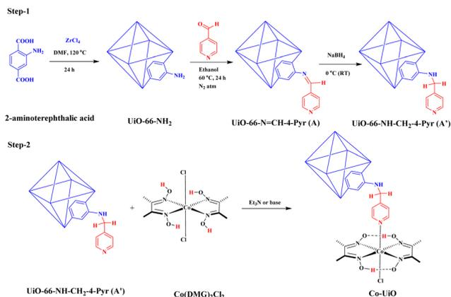
Fig. 1 Synthetic representation for the formation of UiO-66-NH<sub>2</sub> and its post-synthetic modifications with the molecular Co(DMG)<sub>2</sub>Cl<sub>2</sub> complex.
