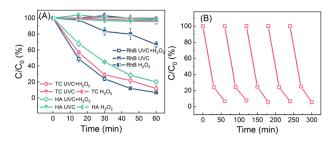
Fig. 4 (A) The removal of RhB, TC and HA via UVC/H<sub>2</sub>O<sub>2</sub>, UVC and  $H_2O_2$  processes in batch tests; and (B) recyclability of the process for RhB removal (RhB, TC or HA: 1 mg  $L^{-1}$ ; H<sub>2</sub>O<sub>2</sub>: 10  $\mu$ M).
