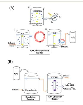
Scheme 1 Schematic illustration of sequencing batch photocatalytic  $H_2O_2$  production over MRF (A) and UVC/ $H_2O_2$  flow-through processes (B) for organic micropollutant degradation.
