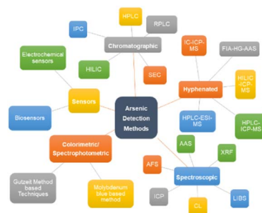
Fig. 3 Different methods of arsenic detection and determination.
