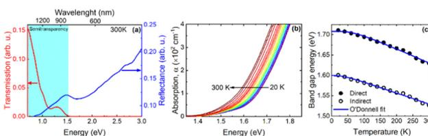
Fig. 6 (a) Room temperature transmission and reflection spectra of bulk NiGa<sub>2</sub>S<sub>4</sub>. (b) Temperature dependence of the absorption spectra of bulk NiGa<sub>2</sub>S<sub>4</sub> in the vicinity of the absorption edge. (c) Temperature dependence of the indirect and direct energy gap for bulk NiGa<sub>2</sub>S<sub>4</sub> determined from absorption measurements.
