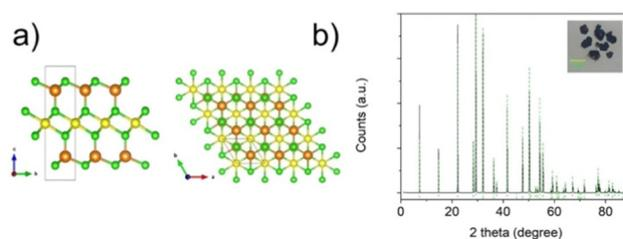
Fig. 1 Crystalline structure of hexagonal  $NiGa_2S_4$  along the  $c$ -axis and the  $ab$  plane. (b) XRD pattern of  $NiGa_2S_4$  crystalline powder. In the inset a sample of the crystals obtained *via* CVT synthesis is shown. The indexed XRD pattern of the  $NiGa_2S_4$  crystals and powders are shown in Fig. S1 and S2 (ESI<sup>†</sup>), respectively.
