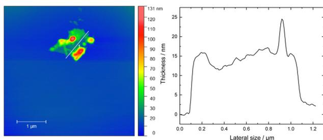
Fig. 4 AFM image and the corresponding height profile plot of exfoliated NiGa<sub>2</sub>S<sub>4</sub>.
