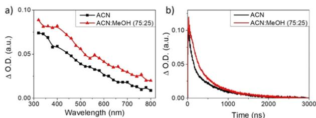
Fig. 9 (a) Transient absorption spectra of the NiGa<sub>2</sub>S<sub>4</sub> dispersion in acetonitrile (black) and acetonitrile:ethanol (75 : 25, v/v) (red) at 500 ns under a N<sub>2</sub> atmosphere upon 420 nm laser excitation. (b) Transient absorption decay of NiGa<sub>2</sub>S<sub>4</sub> dispersion in acetonitrile (black) and acetonitrile:ethanol (75 : 25, v/v) (red) monitored at 560 nm under a N<sub>2</sub> atmosphere upon 420 nm laser excitation.
