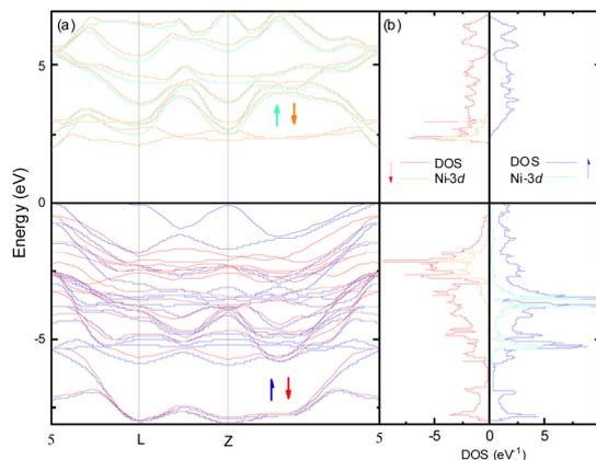
Fig. 2 Calculated electronic structure of  $\text{NiGa}_2\text{S}_4$ . (a) Band structure along principal directions of the first Brillouin zone. (b) Density of states (DOS) for the spin-up ( $\uparrow$ ) and spin-down ( $\downarrow$ ) channels including PDOS for Ni-3d states.
