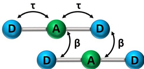
Fig. 5 A sketch of intramolecular ( $\tau$ ) and intermolecular ( $\beta$ ) charge resonance interactions, shown as double-sided arrows, for a pair of adjacent molecules.
