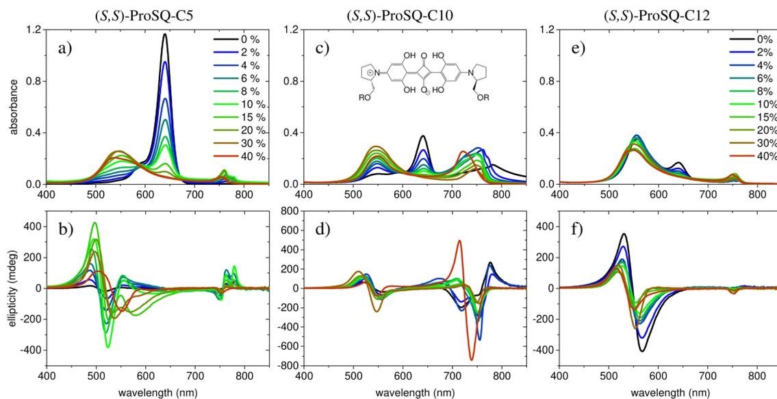
**Fig. 1** Experimental UV/Vis absorbance spectra (top row) and corresponding ellipticity spectra (bottom row) for selected (*S,S*)-ProSQ compounds with varying alkyl chain lengths: C5 in (a and b), C10 in (c and d), and C12 in (e and f). The inset in (c) sketches the molecular structure where R denotes the varying alkyl chain. The legend indicates the volume-percentage of water in the methanol–water mixture and applies to all plots.
