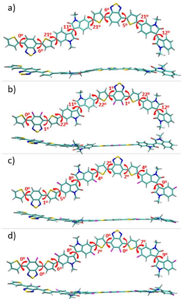
Fig. 2 Top and lateral views of the optimized geometries (at the B3LYP/6-31G\*\* level of theory) for the dimeric models of **P1** (a), **P2** (b), **P3** (c) and **P4** (d) polymers. The dihedral angle values between selected rings are also shown.
