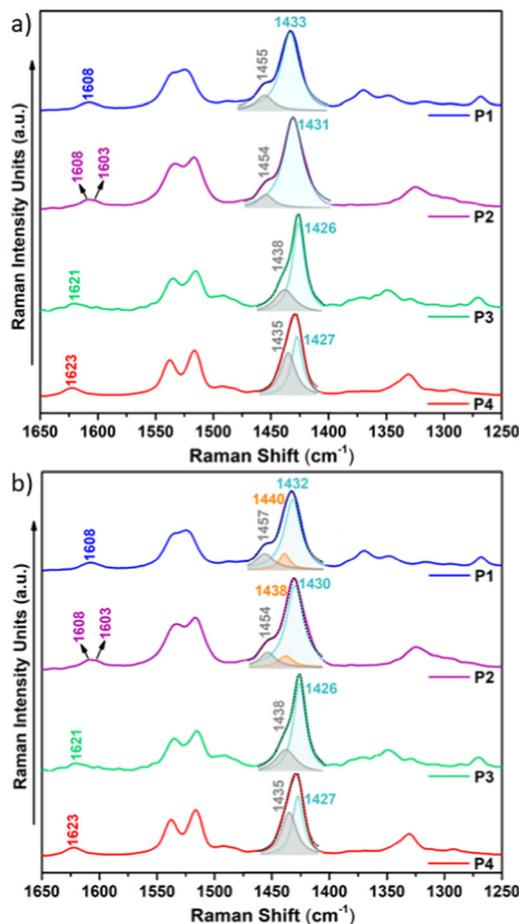
Fig. 10 Solid-state FT-Raman spectra ( $\lambda_{\text{exc}} = 1064 \text{ nm}$ ) of copolymers **P1**–**P4** with (a) a simple two-component deconvolution of representative Raman bands and (b) the optimal deconvolution which best fits the experimental data.
