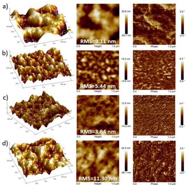
Fig. 9  $1 \times 1 \mu\text{m}^2$  tapping-mode AFM images of 3D-topography (left), height (middle) and phase (right) for (a) **P1**, (b) **P2**, (c) **P3** and (d) **P4** films prepared under optimal device performance conditions. The corresponding root-mean-square (RMS) roughness is also shown.
