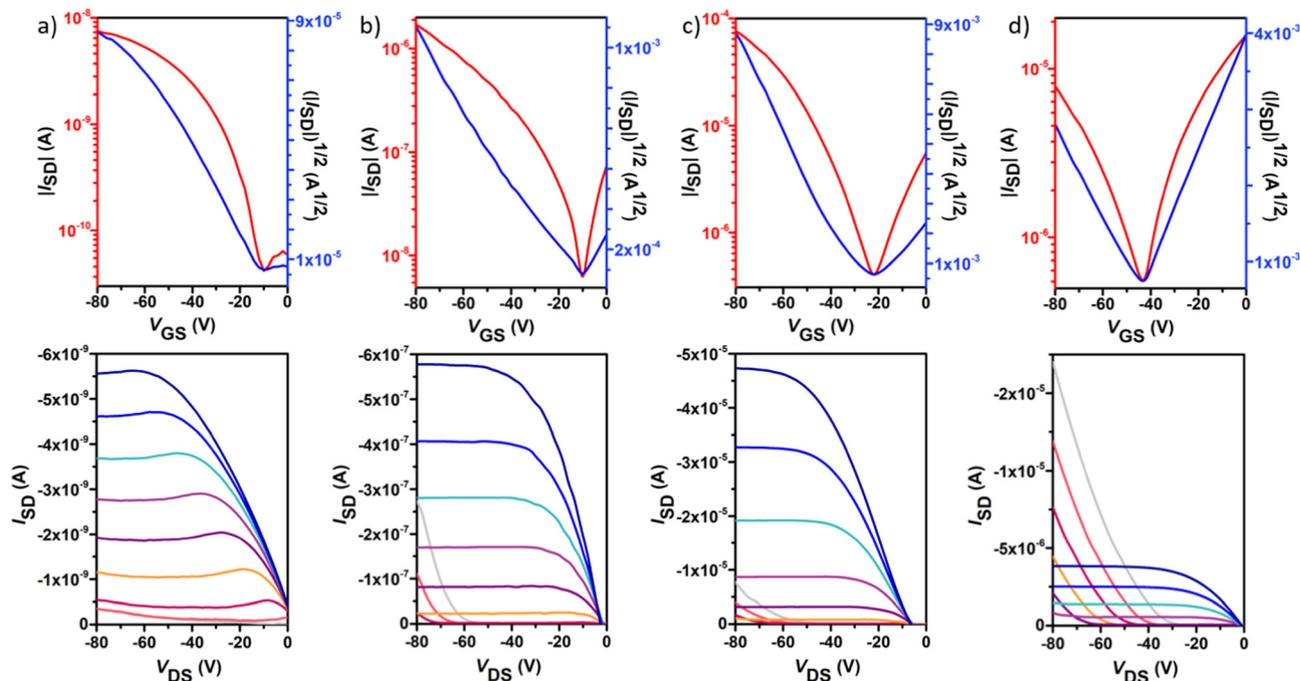
Fig. 6 Typical p-type field-effect transistor transfer (top) and output (bottom) characteristics for polymers **P1** (a), **P2** (b), **P3** (c) and **P4** (d). The transfer characteristics were measured at a source–drain voltage ( $V_{DS}$ ) of  $-80$  V. The output curves were measured at gate voltages ( $V_G$ ) from  $0$  to  $-80$  V in intervals of  $10$  V and over a  $V_{DS}$  range of  $0$  to  $-80$  V.
