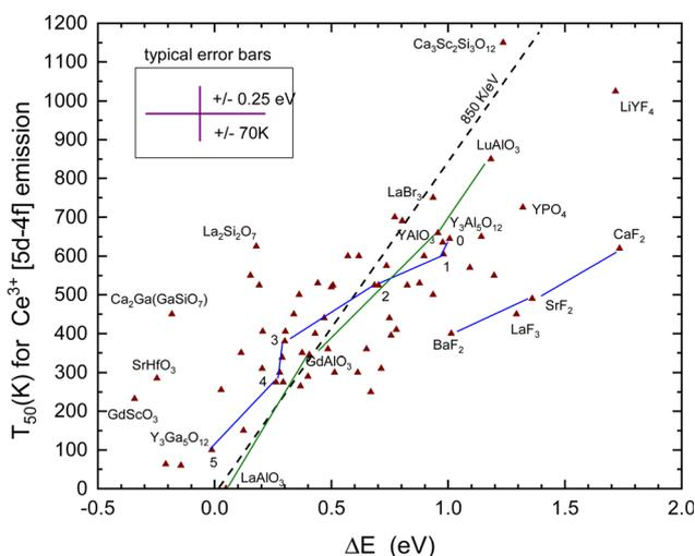
Fig. 8  $T_{50}$  quenching data of the  $\text{Ce}^{3+}$  5d–4f emission against the energy difference  $\Delta E$  between the relaxed 5d-state and the CB-bottom. The typical error bars are shown. Data points for the sequence of compounds  $\text{Y}_3\text{Al}_{5-x}\text{Ga}_x\text{O}_{12}$  and  $\text{REAlO}_3$  (RE = La, Gd, Y, Lu) are connected by straight line segments.
