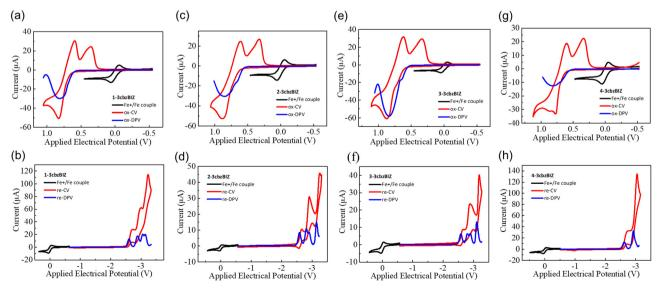
Fig. 3 CV and DPV diagrams of 1-, 2-, 3-, and 4-3cbzBIZs in THF.
