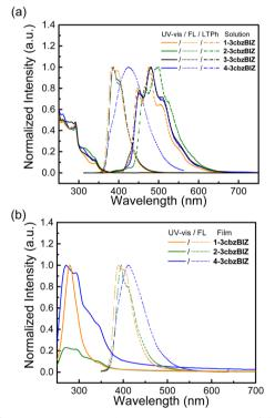
Fig. 5 (a) UV-vis is absorption, fluorescence spectra in THF ( $10^{-5}$  M) and low temperature phosphorescence spectra in Me-THF ( $10^{-5}$  M) at 77 K; (b) UV-vis absorption and fluorescence spectra in thin films.
