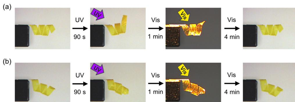
**Fig. 3** Photoinduced deformation behaviours of PAzo/PMMA IPN samples with spiral shapes upon irradiation with UV (365 nm,  $20 \text{ mW cm}^{-2}$ ) and visible light ( $>540 \text{ nm}$ ,  $40 \text{ mW cm}^{-2}$ ). (a) In-plane uniaxial alignment. (b) Homeotropic alignment. Original sizes of the films:  $20 \text{ mm} \times 1 \text{ mm} \times 8 \text{ }\mu\text{m}$ .
