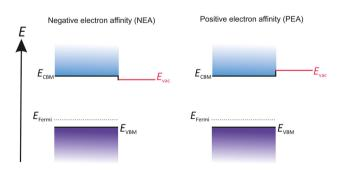
Fig. 4 Comparative illustration of the difference between PEA and NEA surfaces regarding the location of the  $E_{\text{vac}}$ .
