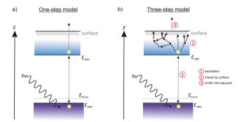
Fig. 2 Comparative illustration of (a) the one-step model and (b) the three-step model.
