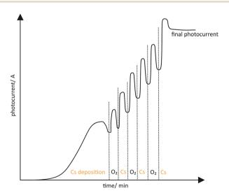
Fig. 9 Schematic drawing of a typical photocurrent evolution when a YoYo activation is used (alternately applying Cs and O2).
