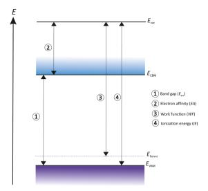
Fig. 1 Schematic representation of the fundamental key terms in photoemission processes.
