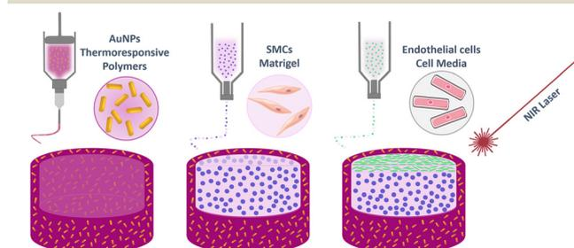
**Fig. 1** Representation of the three printing steps involved in the production of the contractile artery wall model presented. From left to right: first, a thermoresponsive ink is printed forming the base and sides; secondly, SMCs are printed in ECs; and finally, a monolayer of ECs is printed on top.
