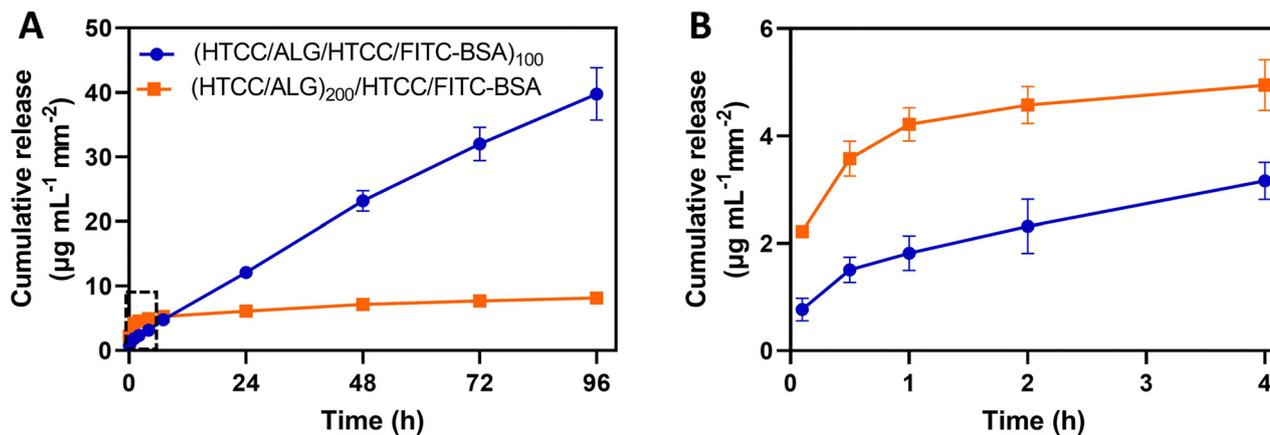
Fig. 9 (A) Cumulative mass release profile of FITC-BSA in PBS at pH 7.4 from (HTCC/ALG/HTCC/FITC-BSA)<sub>100</sub> (blue line and circles) and (HTCC/ALG)<sub>200</sub>/HTCC/FITC-BSA (orange line and squares) FS membranes over 96 h. (B) Zoom-in on the cumulative release of FITC-BSA for the first 4 h (represented with a dotted line in A). Data are presented as mean  $\pm$  SD of three independent experiments ( $n = 3$ , per condition) performed in triplicates.
