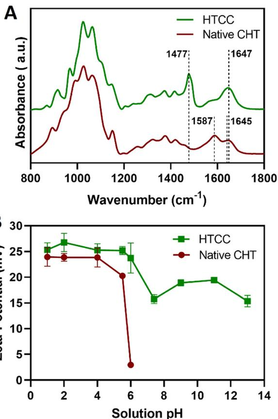
Fig. 4 (A) ATR-FTIR spectra of HTCC and native CHT powders. (B) Evolution of the  $\zeta$ -potential for  $0.1 \text{ mg mL}^{-1}$  HTCC and CHT aqueous solutions as a function of the solution pH presented as mean  $\pm$  SD of three independent experiments ( $n = 3$ , per condition) performed in triplicates.
