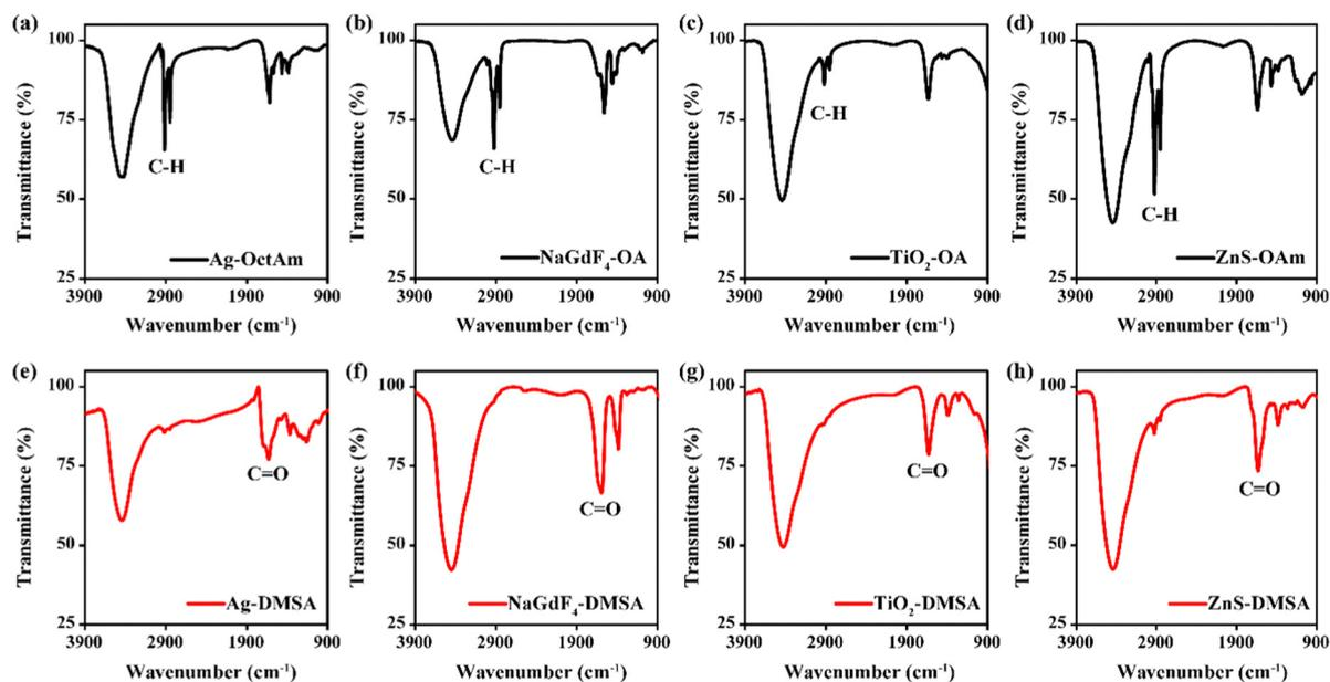
Fig. 4 FTIR spectra of (a) Ag-OctAm, (b) NaGdF<sub>4</sub>-OA, (c) TiO<sub>2</sub>-OA, (d) ZnS-OAm, (e) Ag-DMSA, (f) NaGdF<sub>4</sub>-DMSA, (g) TiO<sub>2</sub>-DMSA and (h) ZnS-DMSA.
