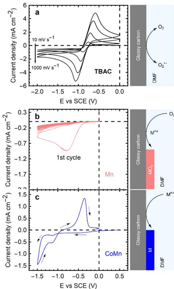
Fig. 1 Current density vs. potential cycles of a GCE in DMF with: (a) 0.1 M TBAC, saturated with oxygen, at scan rates of 10  $\text{mV s}^{-1}$ , 100  $\text{mV s}^{-1}$ , 500  $\text{mV s}^{-1}$ , 1000  $\text{mV s}^{-1}$ . (b) 0.1 M  $\text{MnCl}_2$  saturated with oxygen, at 50  $\text{mV s}^{-1}$ . (c) 0.05 M  $\text{CoCl}_2$ , 0.05 M  $\text{MnCl}_2$ , de-oxygenated, at 50  $\text{mV s}^{-1}$ . Sketches of the respective processes accompany the curves.
