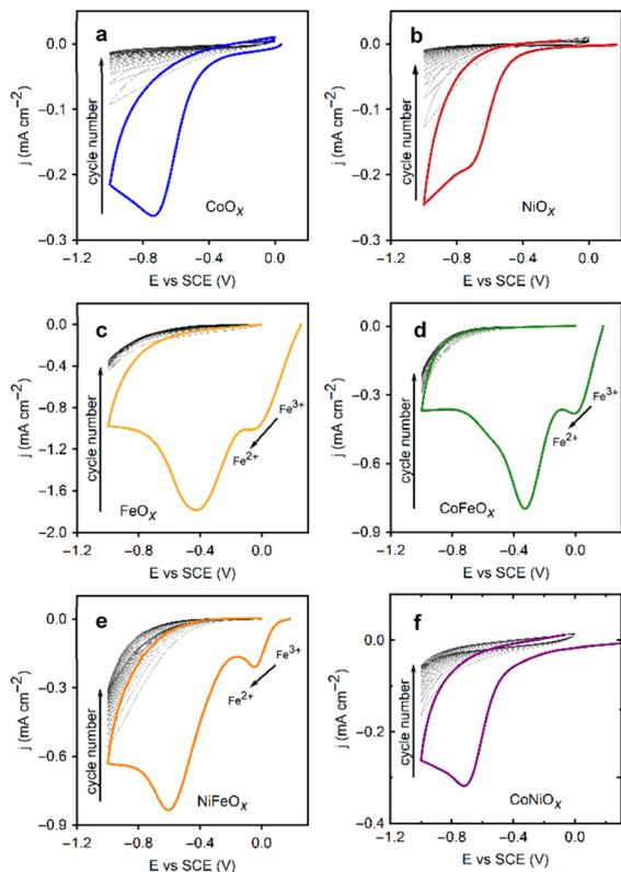
Fig. 3 Cyclic voltammograms at  $20 \text{ mV s}^{-1}$  of the deposition of the single (Ni, Co, Fe) and mixed (CoFe, NiFe, CoNi) metal oxides over 20 cycles. Potential regions for the electrochemical reactions discussed are noted. The cycle number increases from each initial cycle highlighted, to the subsequent cycles trending towards 0 current. (a) Co. (b) Ni. (c) Fe. (d) CoFe. (e) NiFe. (f) CoNi.
