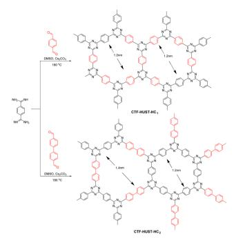
Fig. 15 Synthesis of CTF-HUST-HC<sub>1</sub> and CTF-HUST-HC<sub>2</sub>.
