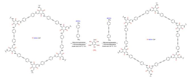
Fig. 5 Synthesis of TP-EDDA and TP-BDDA COFs.
