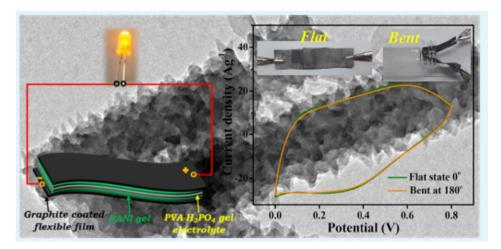
Fig. 22 Flexible supercapacitor assembled with  $MoS_2$  quantum dot (QD)/PANI hydrogel electrodes and  $PVA/H_2SO_4$  gel electrolyte, reproduced with permission from ref. 179 with permission from the American Chemical Society.
