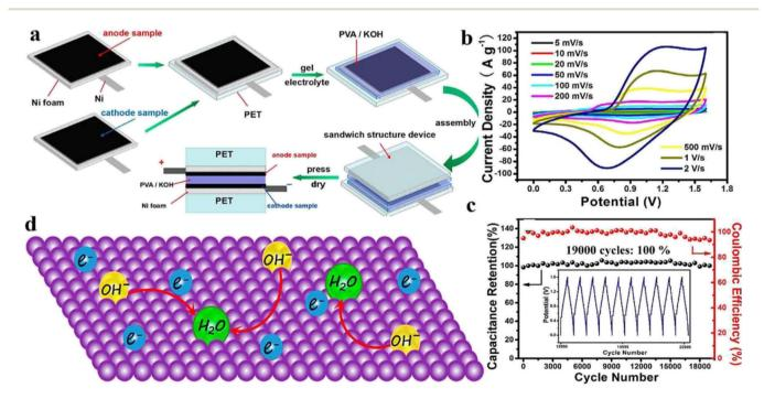
Fig. 23 The flexible supercapacitor device performance. (a) The preparation progress of the device. (b) CV curves at various scan rates in PVA/ KOH gel electrolyte system. (c) Cycling performance and coulombic efficiency of the all-solid ASC at current density of 2 A  $g^{-1}$ ; (d) schematic illustration of the energy storage mechanism on monolayer Ni, Co-HC. Reproduced from ref. 232 with permission from the American Chemical Society.
