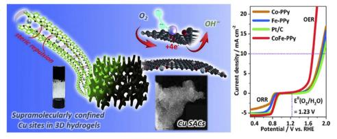
Fig. 9 Hydrogels for electrocatalysis. (a) Hydrogel-derived confined atomic Cu(ı)—N sites and (b) Co/Fe-PPy for electrocatalytic OER and ORR. (Reproduced with from ref. 74 and 75 with permission from Elsevier and American Chemical Society).
