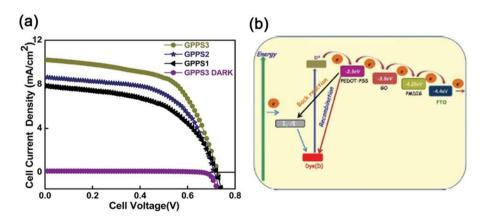
Fig. 2 (a) Plot of J-V characteristics of GPPS1, GPPS2 and GPPS3 under AM 1.5G light illumination of 100 mW cm<sup>-2</sup>. (b) Energy level diagram of the components of GPPS gels explaining the photocurrent behavior of the FTO/GPPS gel/graphite DSSC with the N719 dye. Reproduced from ref. 20 with permission from the Royal Society of Chemistry.
