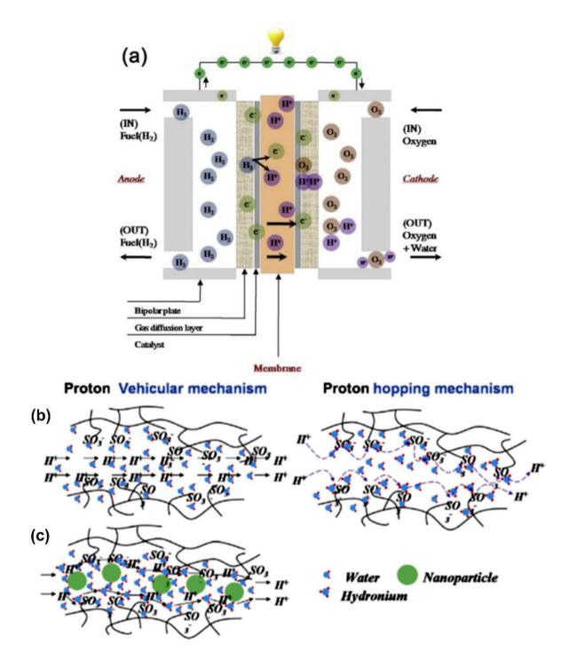
Fig. 6 (a) Principle of polymer electrolyte membrane fuel cell. Schematic design of vehicular mechanism and hopping mechanism as proton conduction in (b) pristine membranes and (c) polymer/nano-particle composite membranes reproduced from ref. 54 with permission from Elsevier.
