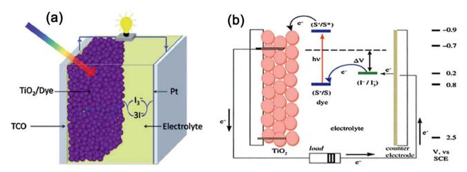
Fig. 1 (a) A schematic diagram of a DSSC device, (b) working principle of a DSSC showing the sequence of electron transfer. Reproduced from ref. 16 with permission from the Royal Society of Chemistry
