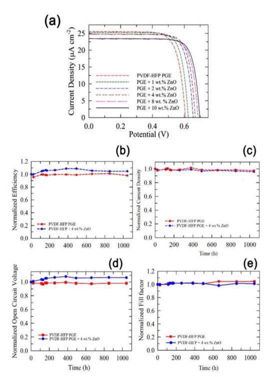
Fig. 4 (a) J-V curves of the QS-DSSCs using PVDF-HFP PGEs with and without various concentrations of ZnO nanofillers. (b) Normalized efficiency, (c)  $J_{sc}$ , (d)  $V_{oc}$ , and (e) FF of the QS-DSSC with and without 4 wt% ZnO nanofillers under continuous light illumination of 200 lx at 35 °C. (Reprinted from ref. 47 with permission from American Chemical Society).
