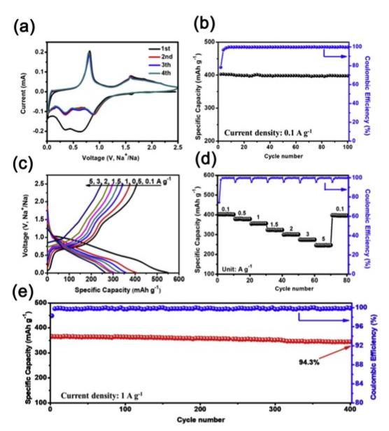
Fig. 17 (a) CV curves of NiSb@3DCM anode at a scan rate of  $0.1 \text{ mV}^{-1}$  for the first four cycles. (b) Cycling performance of NiSb@3DCM anode at 0.1 A g<sup>-1</sup>. (c) Discharge/charge profiles of NiSb@3DCM anode at different current densities from 0.1 to 5 A g<sup>-1</sup> and (d) the corresponding rate performance. (e) Cycle stability of NiSb@3DCM at  $1.0 \text{ A g}^{-1}$ . Reproduced from ref. 132 with permission from Elsevier.
