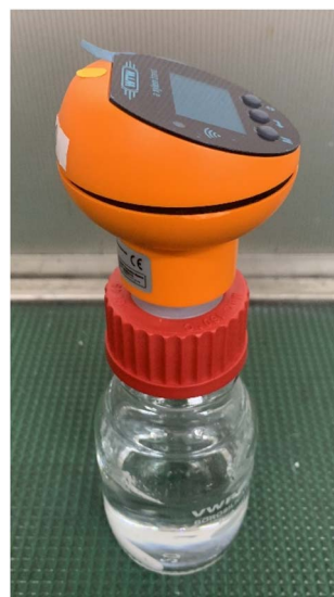
Fig. 3 Commercial biodegradability measuring machine.
