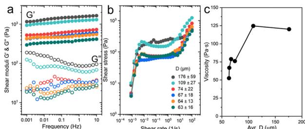
Fig. 2 Rheological characterization of jammed PAAm microgel suspensions. (a) Small amplitude oscillatory frequency sweeps that determine  $G'$  (solid circles) and  $G''$  (hollow circles). (b) Shear rate sweeps that determine the yield stress of PAAm microgel suspensions. (c) Viscosity at  $1.0 \text{ s}^{-1}$  for PAAm microgel suspensions with different average  $D$ .
