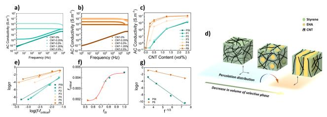
Fig. 3 AC conductivity of (a) PS/MWCNT and (b) P(St-b-EHA)/MWCNT (P6) composite films between 1 Hz-1 MHz, (c) conductivity at 10 Hz for composites as a function of CNT content. (d) Schematic representation of possible CNT particle distribution forming percolation with changing phasetype. (e) Logarithmic plot of conductivity versus reduced CNT content, (f) relation between percolation threshold ( $f_{Critical}$ ) and  $f_{St}$ , and (g) relation between conductivity per unit volume styrene.
