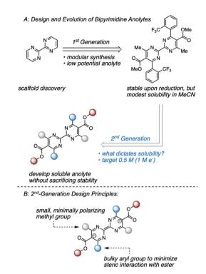
Fig. 1 (A) Evolution of bipyrimidine anolytes. (B) Design principles of 2nd-generation candidates aimed at maintaining a stable reduced state.
