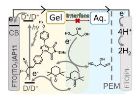
Fig. 29 Photoelectrochemical cell for glycerol oxidation and simultaneous H2 evolution proposed by Reek and co-workers. At the photoanode, the yellow and azure colours represent the redox-gel layer and the aqueous solution, respectively, while oxidation of glycerol by oxoammonium TEMPO+ occurs at the interface (green area). Reprinted from ref. 156 with permission from Wiley, copyright 2022.
