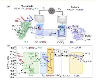
Fig. 3 (a) Representation of the photoelectrochemical cell developed by Reisner and co-workers for bias-free water oxidation and carbon dioxide reduction to formate. The photoanode is an IO-TiO<sub>2</sub>|dpp|P<sub>Os</sub>-PSII photoelectrode, while the cathode is an IO-TiO<sub>2</sub>|FDH. (b) Energy diagram. Reprinted from ref. 65 with permission from the American Chemical Society, copyright 2018
