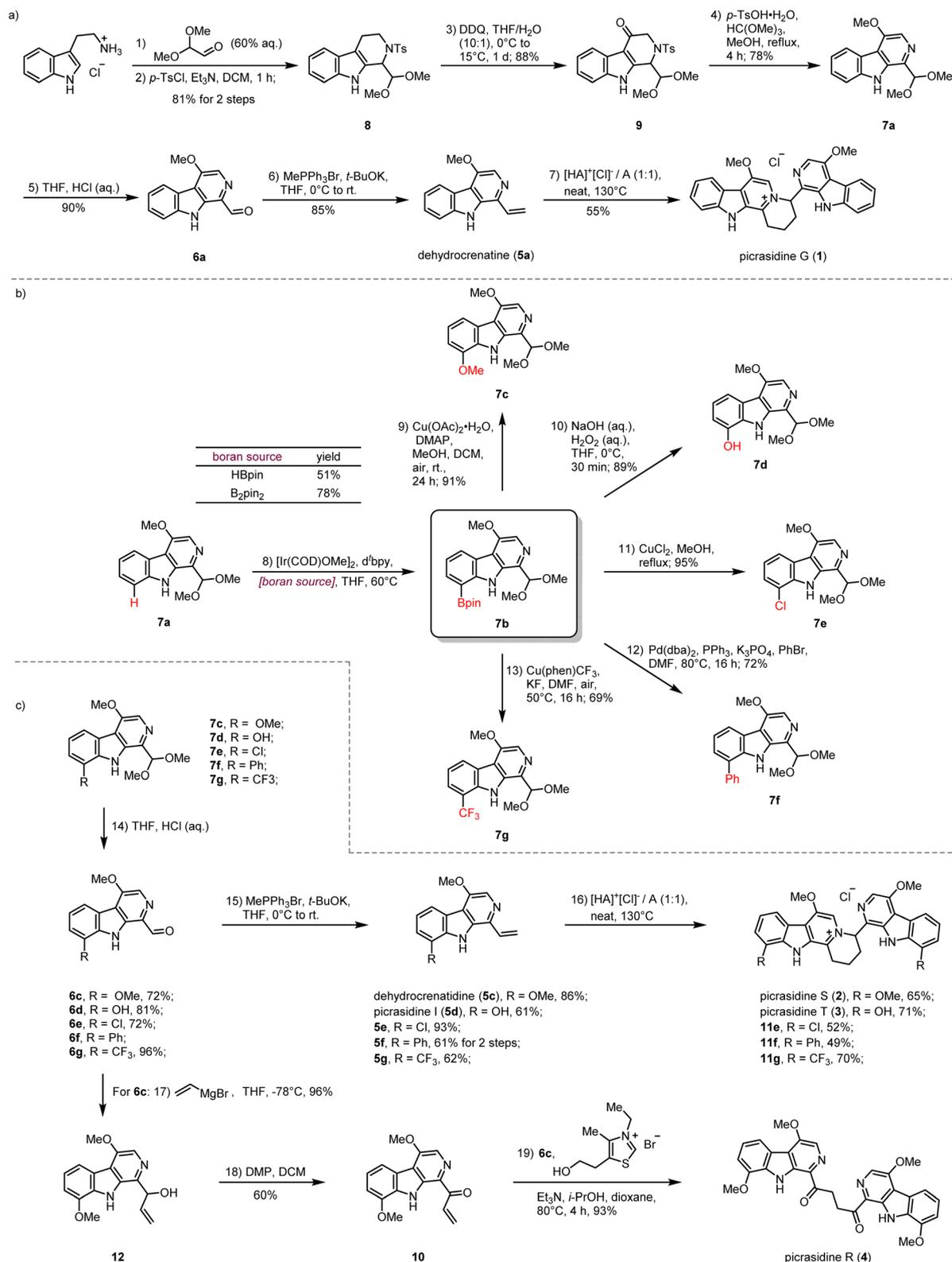
**Scheme 2** (a) Syntheses of picrasidines G (1) by the aza-[4 + 2] cycloaddition. (b) Late-stage C–H functionalization strategy for diversity-oriented syntheses of C-8 substituted  $\beta$ -carboline alkaloids. (c) Total syntheses of picrasidines S (2), T (3), R (4) and 11e, 11f, 11g.
