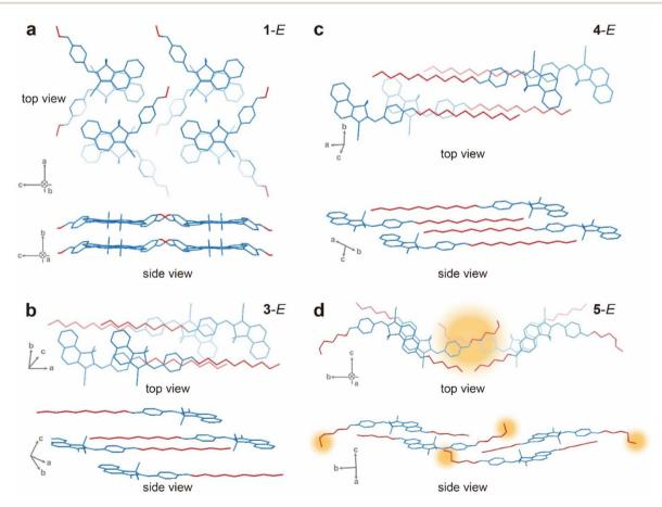
Fig. 4 Crystal structures of (a) 1-E, (b) 3-E, (c) 4-E, and (d) 5-E displayed in two perspectives: top view (top) and side view (bottom). Azo-BF<sub>2</sub> chromophores are coloured in blue, functional groups (R<sub>1</sub> and R<sub>2</sub>) in red, and hydrogen atoms are omitted for clarity. Note: high quality crystals of 2-E were not obtained.
