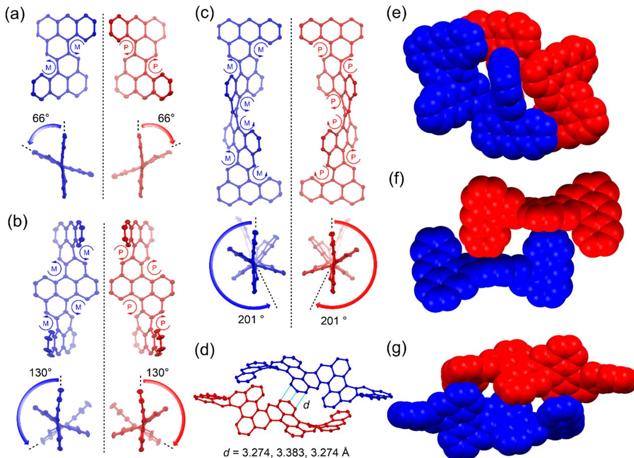
Fig. 2 X-ray crystallographic structures of **1a**, **2a** and **3b**. (a–c) Top view and side view of the crystal structure (backbone only) of **1a**, **2a**, and **3b**, showing 50% probability thermal ellipsoids. (d) Short contacts between the enantiomers of **3b**. (e–g) Illustration of the regular packing pattern of **1a**, **2a**, and **3b**.
