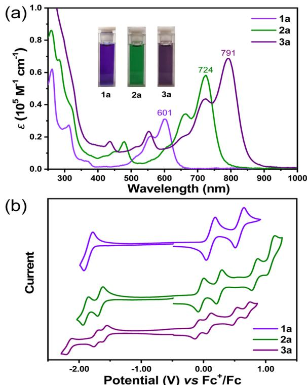
Fig. 3 (a) UV-vis spectra of **1a**, **2a** and **3a** in dichloromethane ( $1 \times 10^{-5}$  M), inset are the photos of their solutions. (b) Cyclic voltammograms of **1a**, **2a** and **3a** (V vs.  $\text{Fc}^+/\text{Fc}$ , in 0.1 M  $\text{nBu}_4\text{N}^+\text{PF}_6^-/\text{dichloromethane}$ ).
