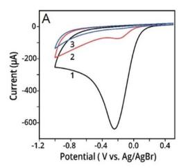
Fig. 12 (A) Three repetitive CV scans of conductive electrode covered with AuNPs-cit in aryldiazonium solution. The scan rate was  $0.1 \, \text{V s}^{-1}$ . (B) Radical electrografting mechanism of diazonium precursor on a conductive electrode surface. Reprinting (adapted) with permission from ref. 150. Copyright 2021, American Chemical Society.
