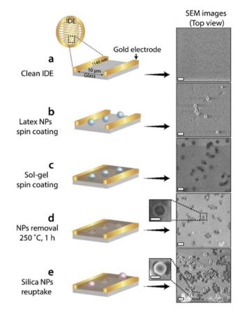
Fig. 16 Schematic illustration of the NAIM-IDE-based approach (left) and the corresponding SEM images (right): (a) a bare IDE; (b) following spin-coated with latex-NPs; (c) upon spin-coated with sol-gel; (d) after removal of the latex NPs; (e) following the reuptake of 100 nm silica NPs. Scale bar: 200 nm. Reprinted (adapted) with permission from ref. 161. Copyright 2022, American Chemical Society.
