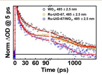
Fig. 7 Normalized kinetic traces of WO $_3$  (black), Ru-UiO-67 (gold), and Ru-UiO-67/WO $_3$  (blue) at 485 nm. Kinetic fits are red traces. The kinetics were normalized at 5 ps to exclude early-time excited state dynamics occurring within [Ru(tpy)(dcbpy)OH $_2$ ] $^{2+}$  (see main text).
