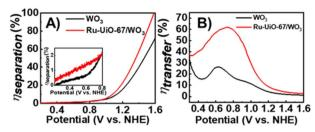
Fig. 5 (A) Charge separation efficiency ( $\eta_{sep}$ ) of WO $_3$  (black) and Ru-UiO-67/WO $_3$  (red) films; inset shows the same figure but magnified from 0.2 to 0.8 V vs. NHE. (B) Charge transfer efficiency ( $\eta_{trans}$ ) for WO $_3$  (black) and Ru-UiO-67/WO $_3$  (red) films. Addition of Ru-UiO-67 to WO $_3$  improves charge separation and charge transfer within WO $_3$  at the electrode surface over all applied potentials.
