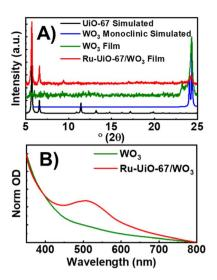
Fig. 1 (A) PXRD patterns of simulated UiO-67 (black), monoclinic  $WO_3$  (red),  $WO_3$  film (blue), and Ru-UiO-67/ $WO_3$  (orange). (B) Ground-state absorption spectra of  $WO_3$  (black), and Ru-UiO-67/ $WO_3$  (red).
