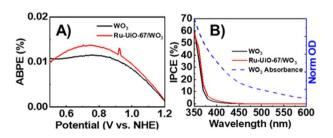
Fig. 3 (A) Photo-response efficiency of WO $_3$  (black) and Ru-UiO-67/WO $_3$  (red) as a function of potential (ABPE). (B) Wavelength (IPCE) of WO $_3$  (black), Ru-UiO-67/WO $_3$  (red) measured under monochromatic light at 500 mV applied potential, overlaid WO $_3$  absorption spectrum (blue dashed line).
