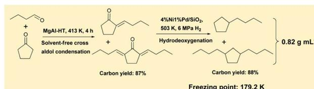
Fig. 13 Condensation reaction of cyclopentanone and butyraldehyde.
