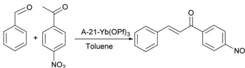
Fig. 3 Condensation reaction of benzaldehyde with *p*-nitroacetophenone.
