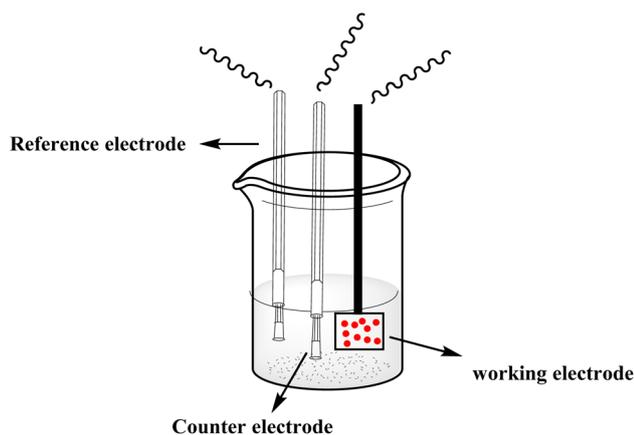
Fig. 2 Electrochemical cell-three electrodes system-of electro-polymerization approach.
