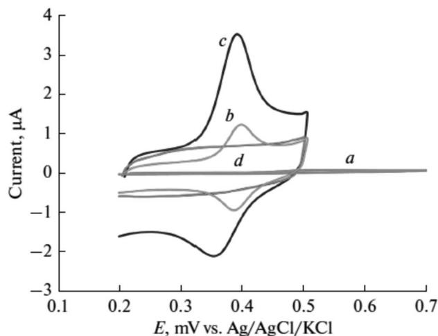
Fig. 23 Cyclic voltammety response of paracetamol (40  $\mu\text{M}$ ) at (a) bare electrode, (b) f-MWCNTs on the electrode, (c) poly(luminol/f-MWCNTs), (d) modified electrode in the absence of paracetamol. This figure has been adapted/reproduced from ref. 59 with permission from Springer Nature via CCC marketplace, copyright (2023).
