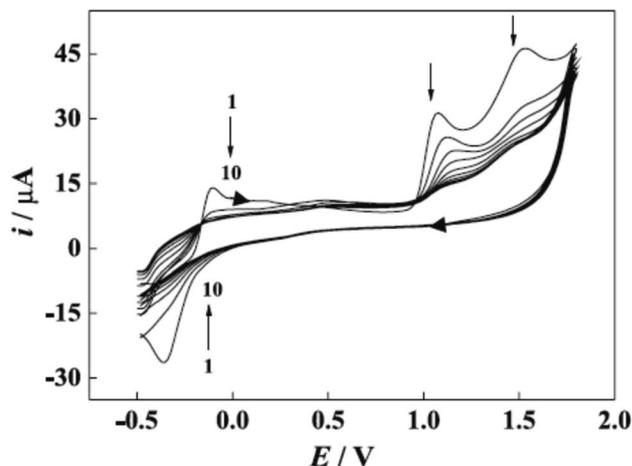
Fig. 3 CV recorded of poly(safranin) electro-polymerization in 0.1 M of sulfuric acid and scan rate:  $50 \text{ mV s}^{-1}$ . This figure has been adapted/reproduced from ref. 6 with permission from PubliSBQ, copyright (2023).
