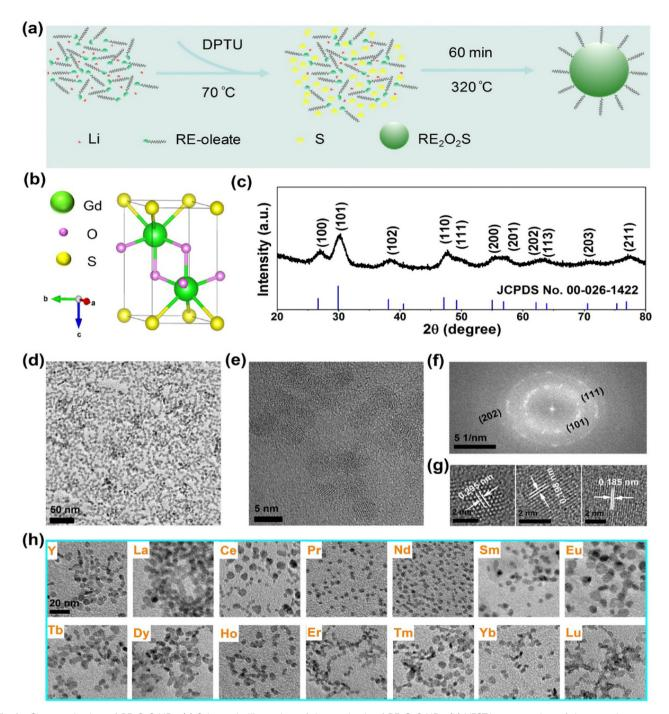
Fig. 1 Characterization of RE<sub>2</sub>O<sub>2</sub>S NPs. (a) Schematic illustration of the synthesis of RE<sub>2</sub>O<sub>2</sub>S NPs. (b) VESTA presentation of the crystal structure of hexagonal Gd<sub>2</sub>O<sub>2</sub>S. (c-g) XRD patterns, typical TEM image, HRTEM image, FFT diffraction and identical planes of Gd<sub>2</sub>O<sub>2</sub>S NPs, respectively. (h) TEM images of 14 kinds of ultrasmall RE<sub>2</sub>O<sub>2</sub>S NPs synthesized by the optimized approach.
