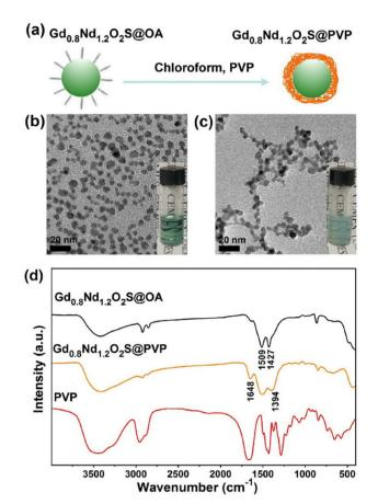
**Fig. 3** Ligand exchange with PVP. (a) Schematic illustration of the synthesis of PVP-coated  $Gd_{0.8}Nd_{1.2}O_2S$  NPs. (b and c) TEM images of OA-coated and PVP-coated  $Gd_{0.8}Nd_{1.2}O_2S$  NPs. Inset photos show the dispersity of nanoparticles in cyclohexane and water with the same concentration of 10 mg mL<sup>-1</sup>, corresponding to before and after ligand exchange, respectively. (d) FTIR spectra of OA-coated, PVP-coated  $Gd_{0.8}Nd_{1.2}O_2S$  NPs and PVP.
