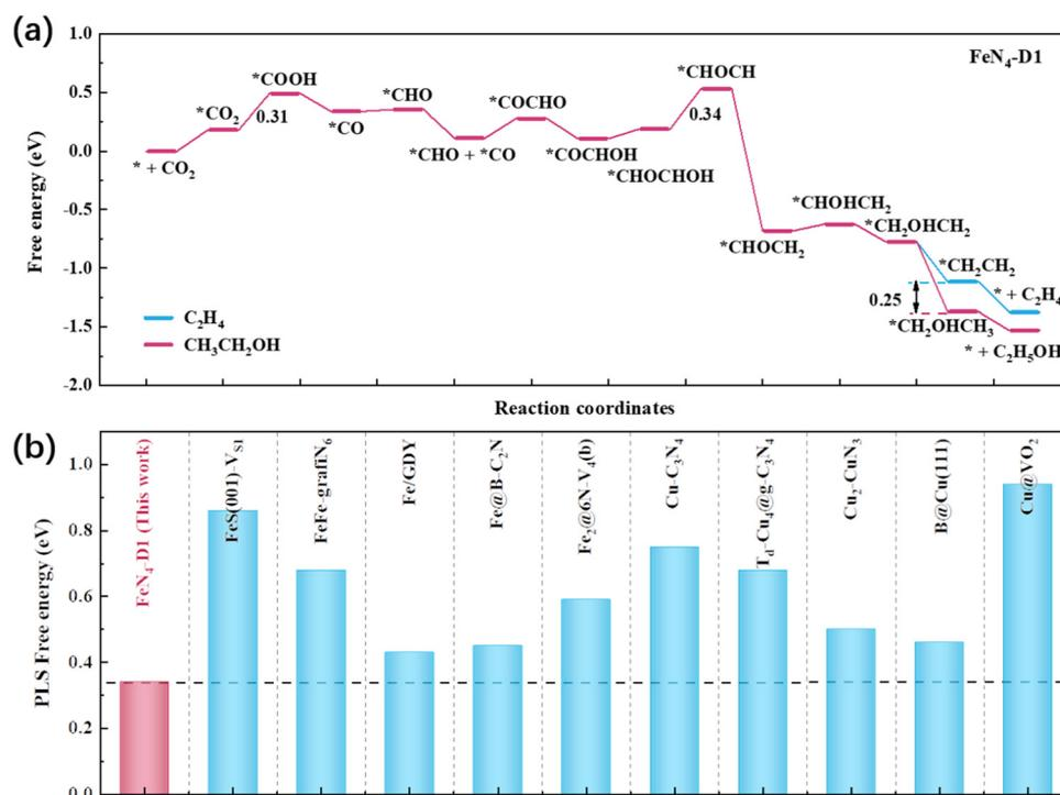
Fig. 5 (a) Reaction free energy profile of CO<sub>2</sub> reduction to C<sub>2</sub>H<sub>4</sub> and C<sub>2</sub>H<sub>5</sub>OH on the FeN<sub>4</sub>-D1 structure. (b) Comparison of the FeN<sub>4</sub>-D1 structure with some reported catalysts on the PLS free energy of C<sub>2</sub>H<sub>5</sub>OH.
