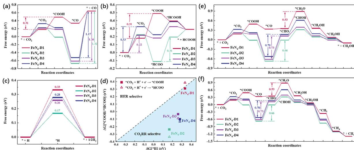
Fig. 3 Reaction free energy profile of CO<sub>2</sub> reduction to CO (a) and HCOOH (b). HER free energy profile (c) and the comparison between the HER and CO<sub>2</sub>RR on the four catalysts (d). Reaction free energy profile of the CO<sub>2</sub>RR to CH<sub>3</sub>OH (e) and CH<sub>4</sub> (f) on FeN<sub>4</sub>-Dx (x = 1, 2, 3, and 4) structures.
