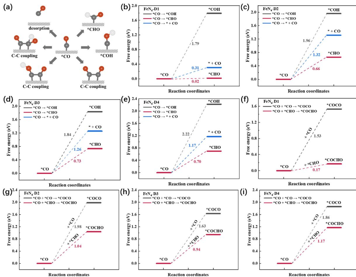
Fig. 4 (a) Schematic diagram of different reaction pathways of the \*CO intermediate. (b–e) Free energy profile of CO desorption and \*CO hydrogenation. (f–i) Comparison of C–C coupling on four FeN<sub>4</sub>-Dx (x = 1, 2, 3, and 4) structures.
