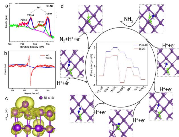
**Fig. 5** (a) Fe 2p XPS of WOF-Au, (b) EPR of WO and WOF-Au,<sup>21</sup> Copyright 2020, American Chemical Society. (c) Partial charge density of the Bi-2B (012) facet, (d)  $N_2$  reduction progress on Bi-2B (012).<sup>72</sup> Copyright 2020, Elsevier.
