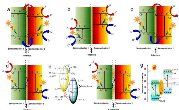
**Fig. 7** Band structure of (a) type I, (b) type II, (c) type III, and (d) Z-scheme heterojunction in semiconductor–semiconductor and for example, (e)  $g-C_3N_4/W_{18}O_{49}$ ,<sup>33</sup> Copyright 2017, the Royal Society of Chemistry. (f) Z-scheme in the semiconductor–electron mediator–semiconductor. A: electron acceptor, D: electron donor; and for example, (g)  $Bi-Bi_2O_3/KTa_{0.5}Nb_{0.5}O_3$ .<sup>88</sup> Copyright 2022, the Royal Society of Chemistry.
