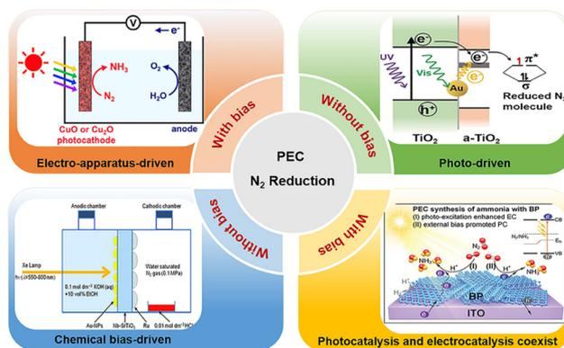
**Fig. 1** Schematic diagram of multiform PEC nitrogen fixation driven by an external bias, solar energy, chemical potential under irradiation, and coexistence of photocatalytic and electrocatalytic  $N_2$  reduction.
