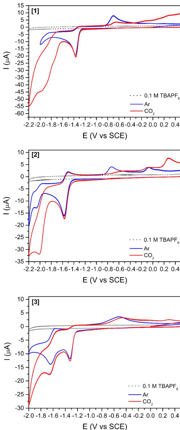
Fig. 2 Cyclic voltammograms of complexes [1], [2], and [3] (1 mM) in DMF, argon, or carbon dioxide saturated solutions using  $\text{TBAPF}_6$  as supporting electrolyte (0.1 M) at  $100 \text{ mV s}^{-1}$ . Glassy carbon (3 mm diameter) was used as working, platinum wire as counter and SCE as reference electrodes.
