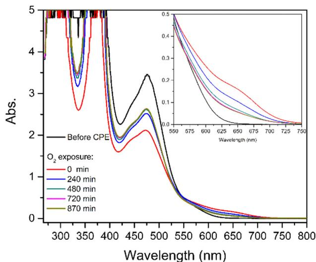
**Fig. 7** UV-vis spectra obtained for [1] after CPE under CO<sub>2</sub> before and during exposure of the solution to atmospheric O<sub>2</sub>.
