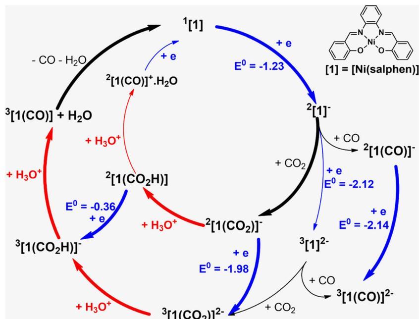
Fig. 9 Pathways for CO<sub>2</sub> reduction to CO in the presence of [Ni(salphen)], [1].
