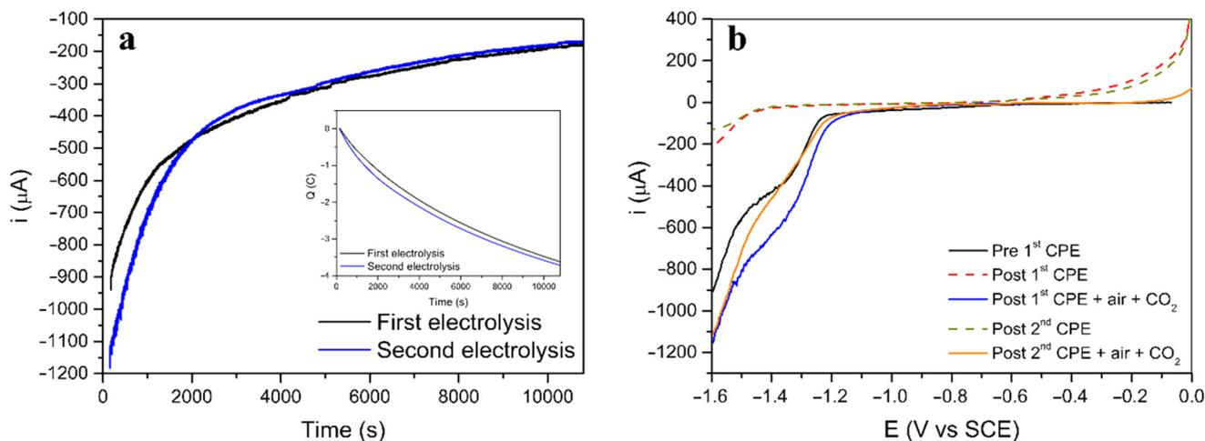
Fig. 4 (a) Current and charge (inset) behavior during both CPE of complex [3]. (b) Linear voltammograms of [3] in DMF using TBAPF<sub>6</sub> as supporting electrolyte (0.1 M) at 10 mV s<sup>-1</sup>. Glassy carbon was used as working electrode, platinum wire as counter and SCE as reference electrode.
