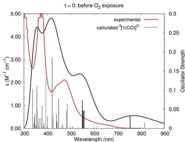
**Fig. 11** Experimental spectrum of the Ni(II)–CO species (red line) and calculated (TDDFT) spectrum of  $^3[1(\text{CO})]^{2-}$  (black line) in DMF. The sticks correspond to the calculated wavelengths. The details of those in bold are given in Table 2.
