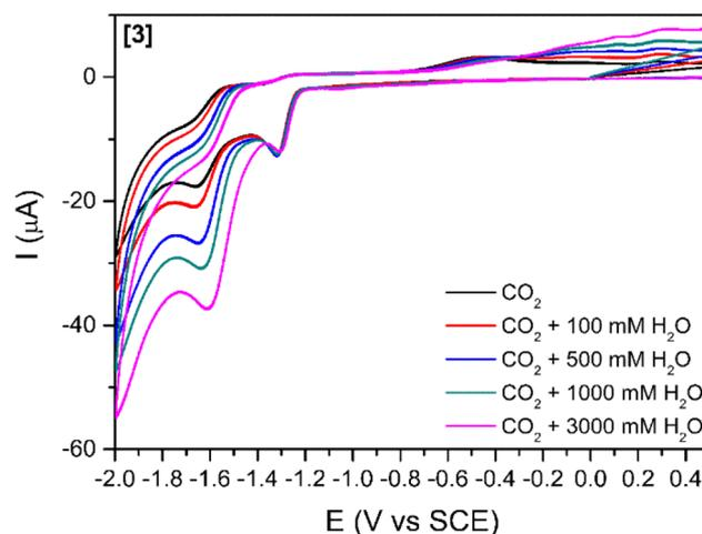
**Fig. 3** Cyclic voltammograms of complex [3] (1 mM) in DMF, carbon dioxide saturated solutions using TBAPF<sub>6</sub> as supporting electrolyte (0.1 M) at 100 mV s<sup>-1</sup>. Effect of different concentrations of added water.
