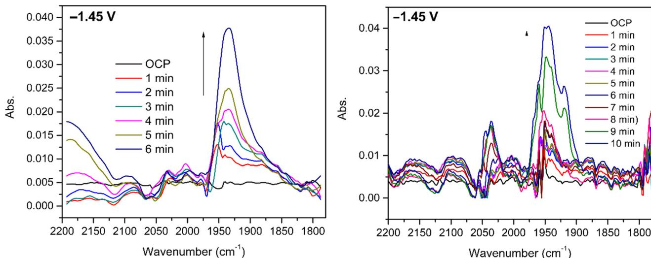
**Fig. 6** SEC-IR experiments at  $-1.45$  V vs. Ag pseudo-reference using 5 mM of [1] and 0.1 M TBAPF<sub>6</sub> in a CO<sub>2</sub> saturated DMF solution, Pt grids as working and counter electrodes and Ag wire as a pseudo-reference electrode: under a CO<sub>2</sub> atmosphere (left); under a CO atmosphere (right).
