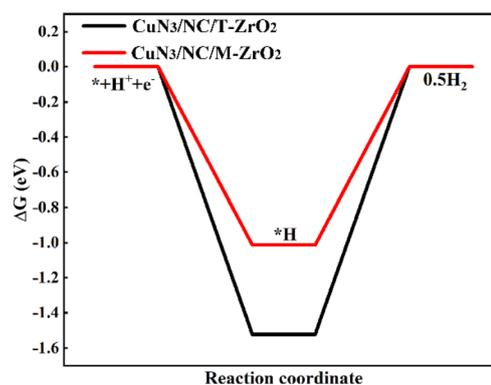
**Fig. 5** DFT-calculated free energy diagrams of the HER on CuN<sub>3</sub>/NC/T-ZrO<sub>2</sub>(101) and CuN<sub>3</sub>/NC/M-ZrO<sub>2</sub>(-111) at a potential (*U*) = 0 V.
