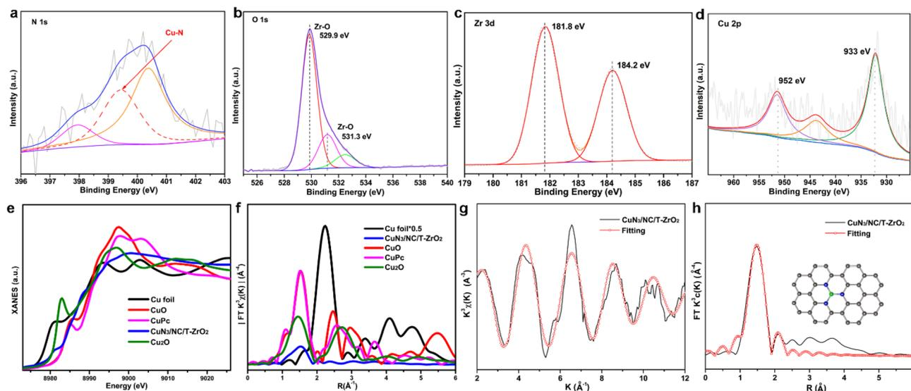
Fig. 2 (a–d) XPS spectra of Cu<sub>3</sub>N<sub>3</sub>/NC/T-ZrO<sub>2</sub>: N 2p, O 1s, Zr 3d, and Cu 2p, respectively. (e) Cu K-edge data of Cu foil, CuO, CuPc, Cu<sub>2</sub>O, and Cu<sub>3</sub>N<sub>3</sub>/NC/T-ZrO<sub>2</sub>. (f) Fourier transform (FT)  $k^3$ -weighted EXAFS profiles at the Cu  $k$ -edge. (g) Fitting curves. (h) EXAFS R space fitting curves of Cu<sub>3</sub>N<sub>3</sub>/NC/T-ZrO<sub>2</sub>.
