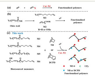
Scheme 1 (a) Palladium-catalyzed copolymerization of ethylene with a polar comonomer. (b) The bioresourced comonomers copolymerized with ethylene. (c) Fabrication of novel polyolefin materials from renewable biomass
