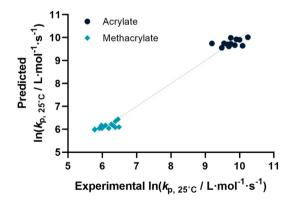
**Fig. 1** The predicted *versus* experimental values of the  $ln(k_p)$  at 25 °C for a dataset containing only meth(acrylates) using the leave one out cross validation on a linear regression. Predictions are determined using a binary indicator whether the monomer is an acrylate (black) or methacrylate (turquoise) and only molecular weight as feature to represent the state-of-the-art in non-ML  $k_p$  predictions ( $r^2 = 0.980$ , RMSE = 0.206).
