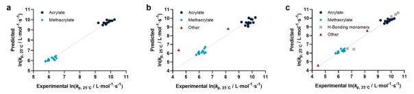
Fig. 3 (a) Comparison of predicted vs. experimental  $\ln(k_p)$  for isolated acrylates and methacrylates ( $r^2 = 0.991$ , RMSE = 0.174), (b) after inclusion of non-meth(acrylate) monomers ( $r^2 = 0.940$ , RMSE = 0.460) and (c) all monomers using available data ( $r^2 = 0.985$ , RMSE = 0.227).
