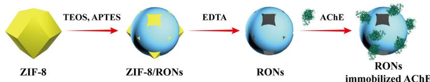
Fig. 2 The preparation process of RONs immobilized AChE.
