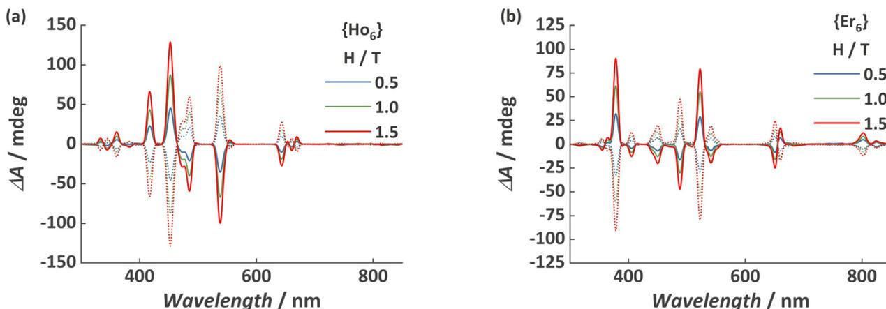
Fig. 1 MCD spectra for (a)  $\{\text{Ho}_6\}$  and (b)  $\{\text{Er}_6\}$  MCAs obtained at  $25^\circ\text{C}$  and under various applied magnetic field. Dotted spectra refer to  $H = -0.5$ ,  $-1.0$ , and  $-1.5 \text{ T}$  magnetic field.
