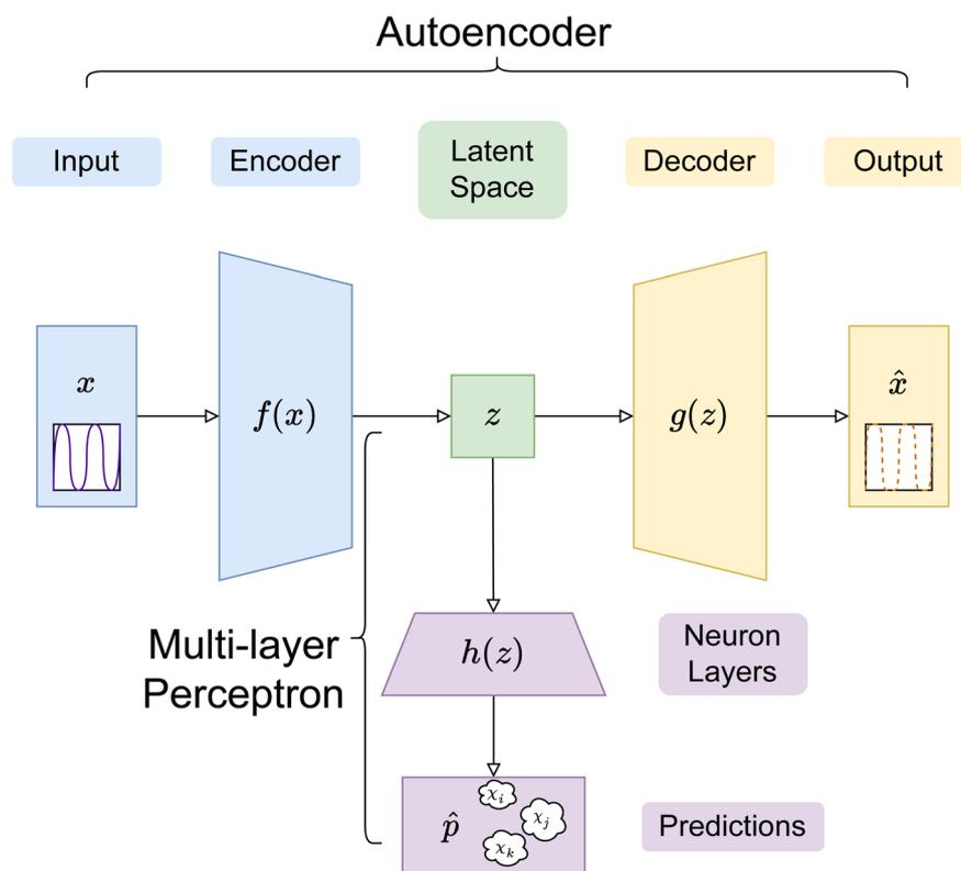
**Fig. 3** Schematic representation of the AE-MLP architecture. The encoder,  $f(x)$ , takes SLD curves,  $x$ , as inputs and compresses them into the latent space,  $z$ . The decoder,  $g(z)$ , generates SLD curves  $\hat{x}$  which, when the AE is properly trained, resemble  $x$ . The multi-layer perceptron (MLP),  $h(z)$ , takes vectors in  $z$  as inputs and outputs the corresponding three Flory–Huggins  $\chi$  parameters.
