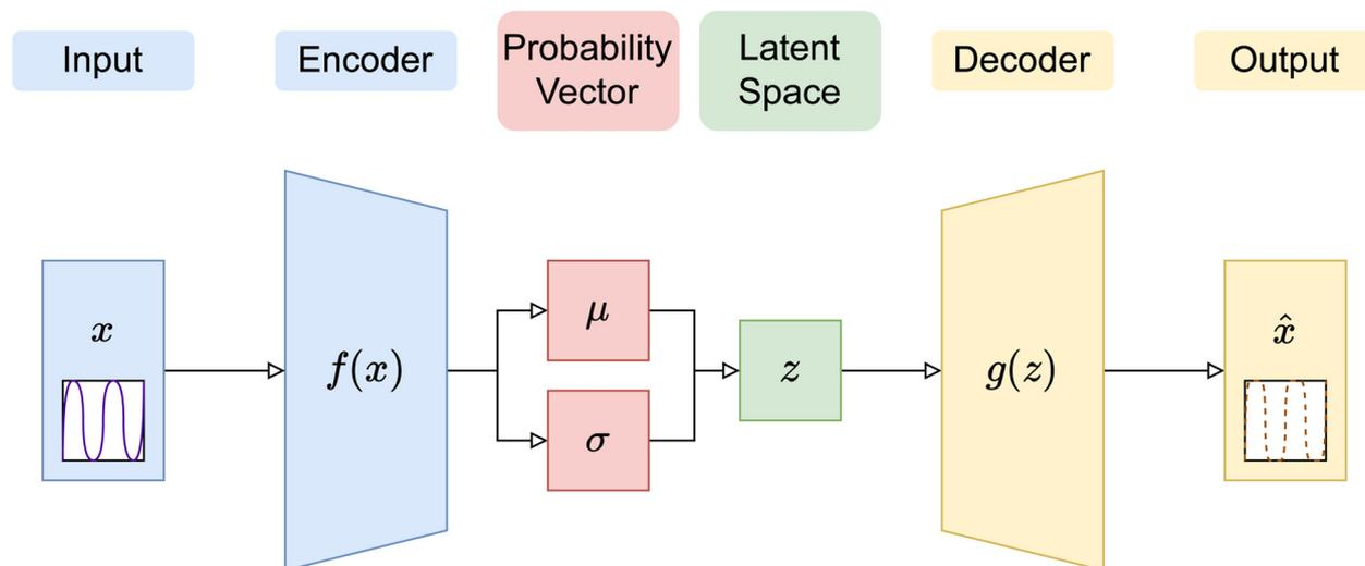
Fig. 4 Diagram of a variational autoencoder (VAE) structure, with the encoding outputs as Bayesian probability vectors shown. All other details are the same as in Fig. 3.
