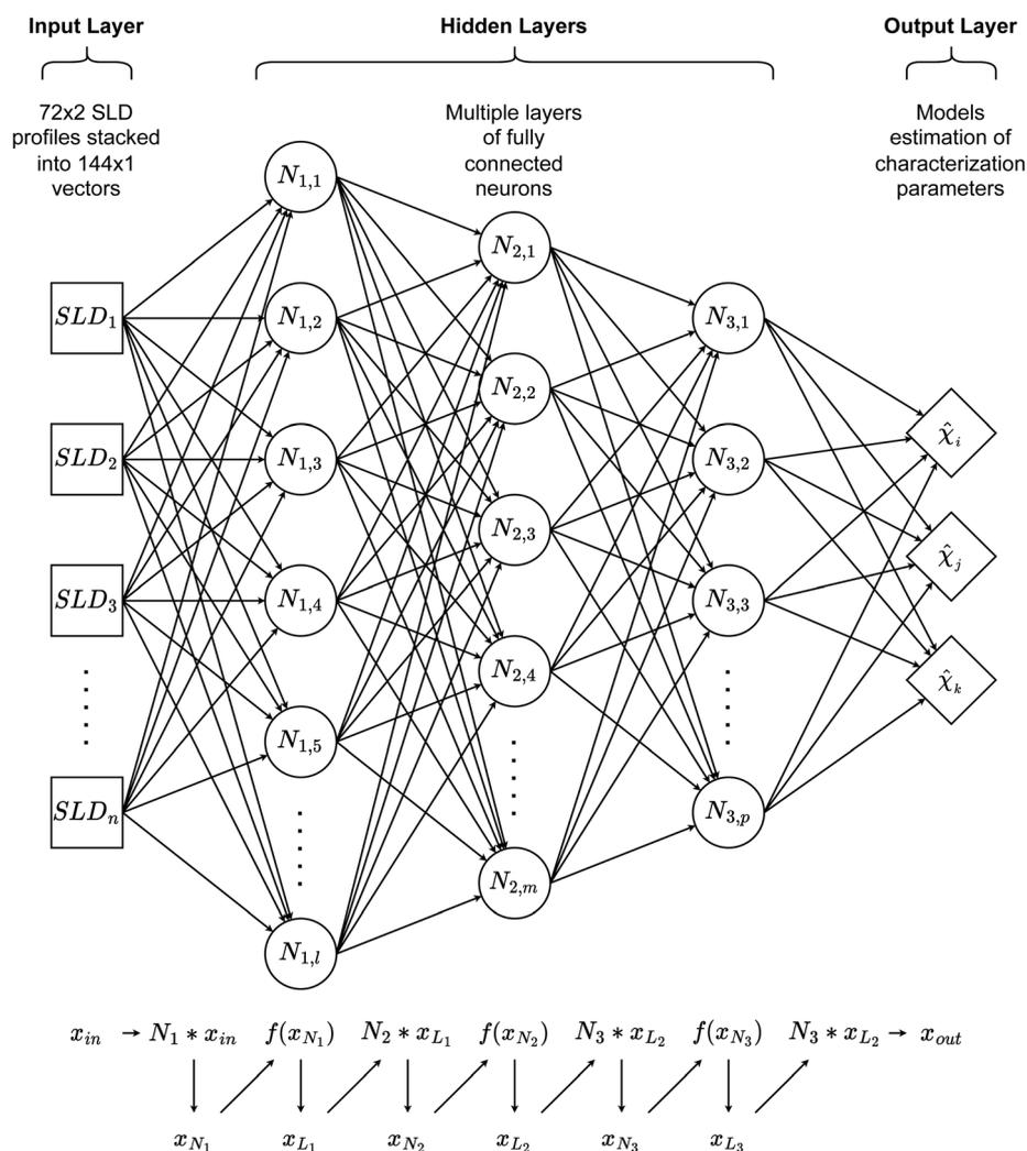
**Fig. 2** Schematic representation of the multi-layer perceptron (MLP) architecture. It takes SLD curves as inputs and outputs the corresponding three Flory–Huggins parameters. Here,  $f(x)$  is an activation function.
