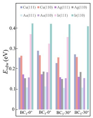
Fig. 3 The vdW interaction between 2D B-G and various metal surfaces with rotation angle of 0° and 30°, respectively.
