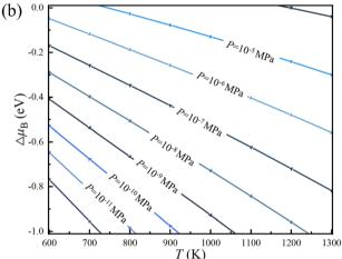
Fig. 5 Chemical potential of (a) carbon and (b) boron under specific experimental parameters of temperature and partial pressure  $(P_{\rm H_2} = 10 \text{ MPa})$ , respectively.
