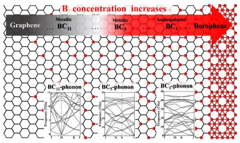
Fig. 1 The structures and calculated phonon spectra of 2D B-G with increased B concentrations (from left to right: BC<sub>11</sub>, BC<sub>5</sub> and BC<sub>3</sub>). The carbon and boron atoms are denoted by the black sticks and red balls, respectively
